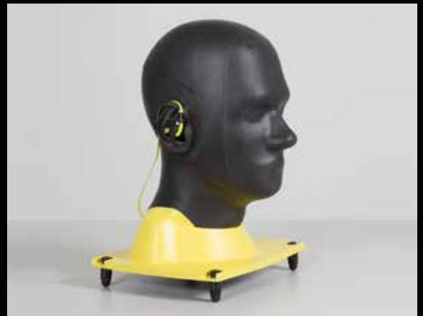
POPEYE10 head phantom in a head-set testing setup
